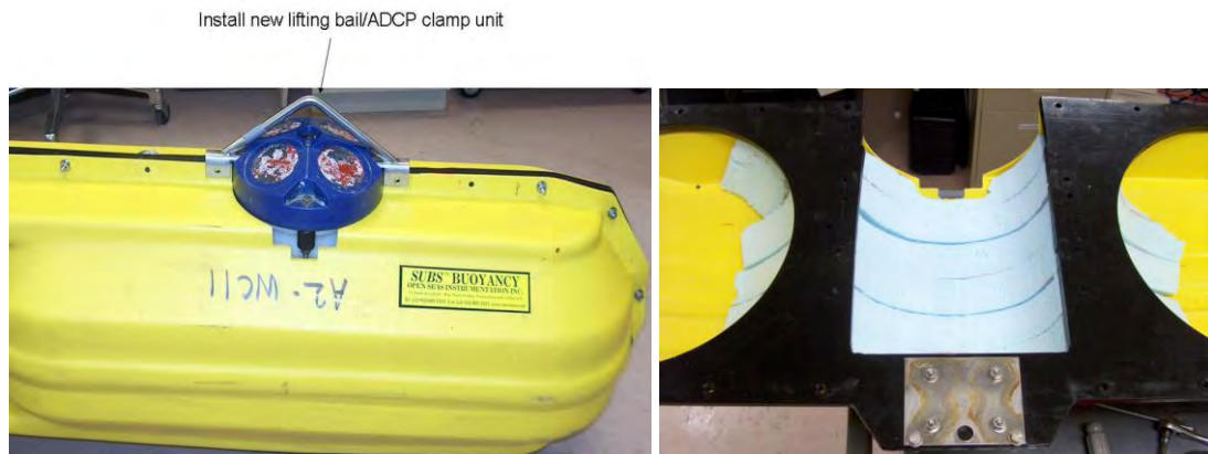
Figure 26. Changes in ADCP installation fixture: New bracket (left), added flotation module (right)
