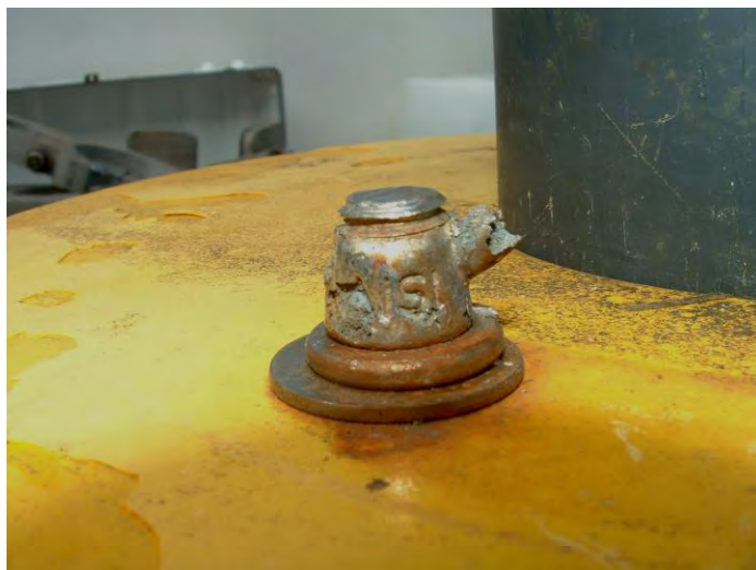
Figure 16. Remains of eye nut after deployment
