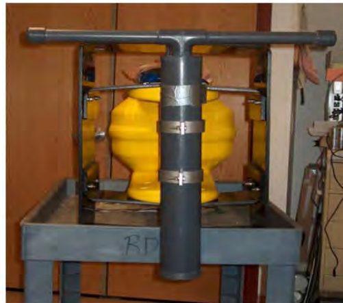
Fig. 7 Argos module attachment (notice its slightly off centered position)
