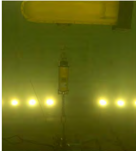
Fig. 9 A2 and dual-CART/chain module (notice its broadside facing the flow)
