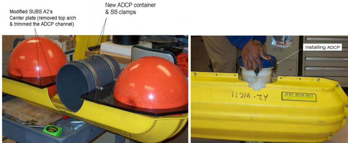
Figure 25. Changes in ADCP installation fixture: ADCP container (left), installing ADCP (right)
