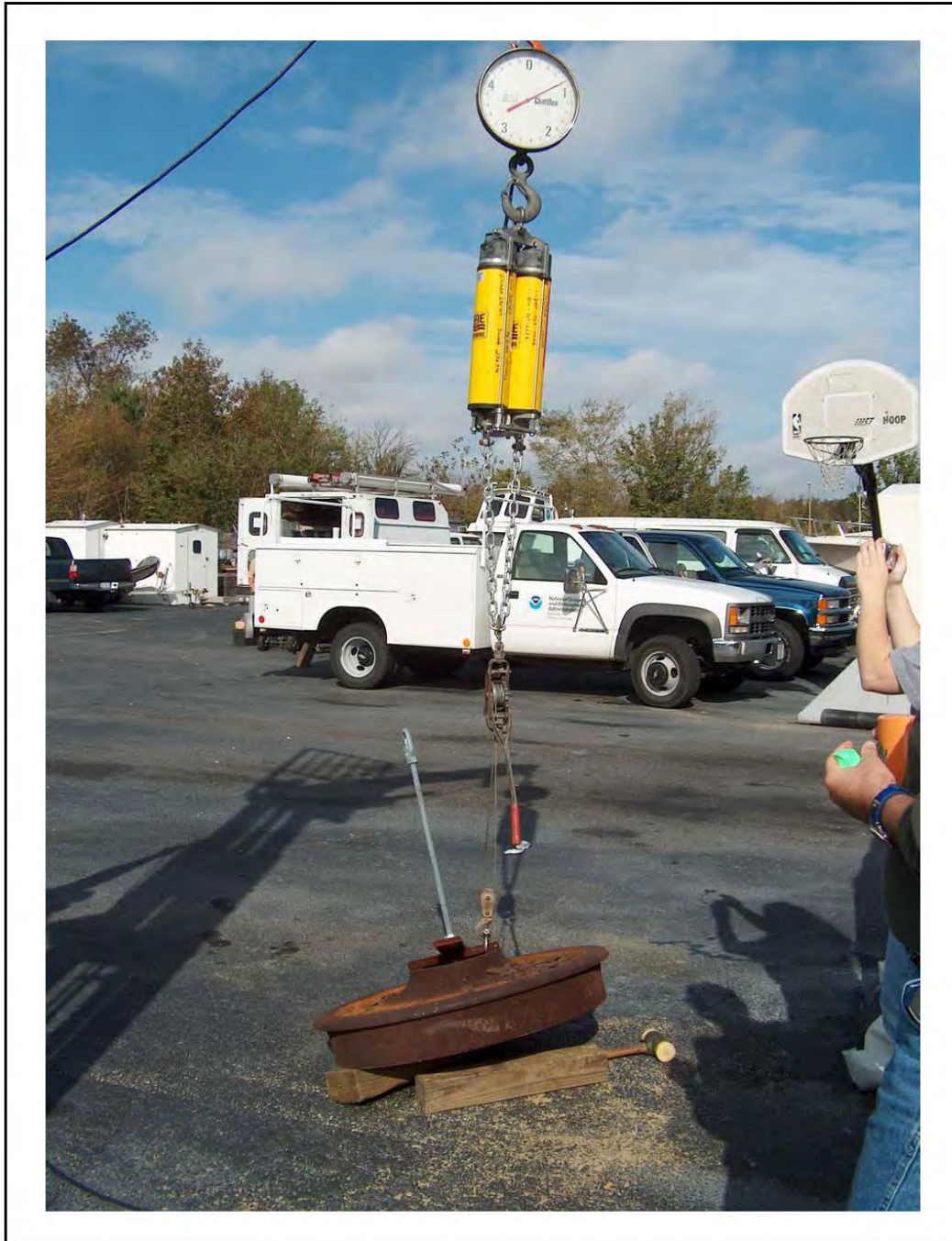
Figure 4. Duel 1 system with 800 lb railroad wheel lifted. Both release shafts are in 'released' position, but the 'old' style pins are hung up.
