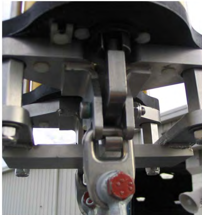
A. CART S/N 30084 @ 200 lbs. Shaft is over rotated.
