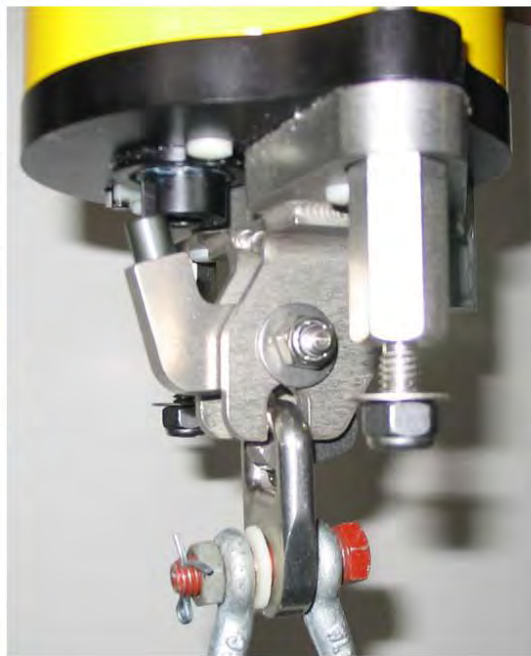
Replaced release shaft which turned properly without any rotation. Old style pin on a single release system. It did not release with railroad wheel off the ground.
