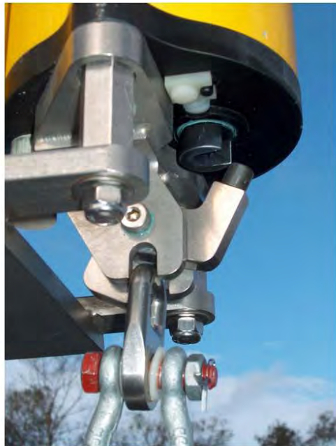
D. CART S/N 30084 @ 800 lbs. Pin is out of shaft but unreleased.
